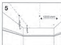
5.Installation of hangers
